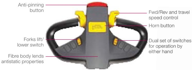
Operator never has to leave the handle during application making operations stable and safe
